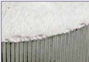
PM with a poor cleanliness The inclusions causes crack initiation and failure
